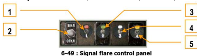
6-49 : Signal flare control panel
