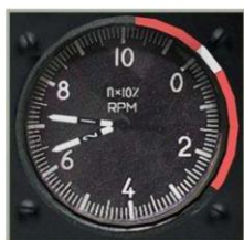
6-26: Engines RPM indicator
